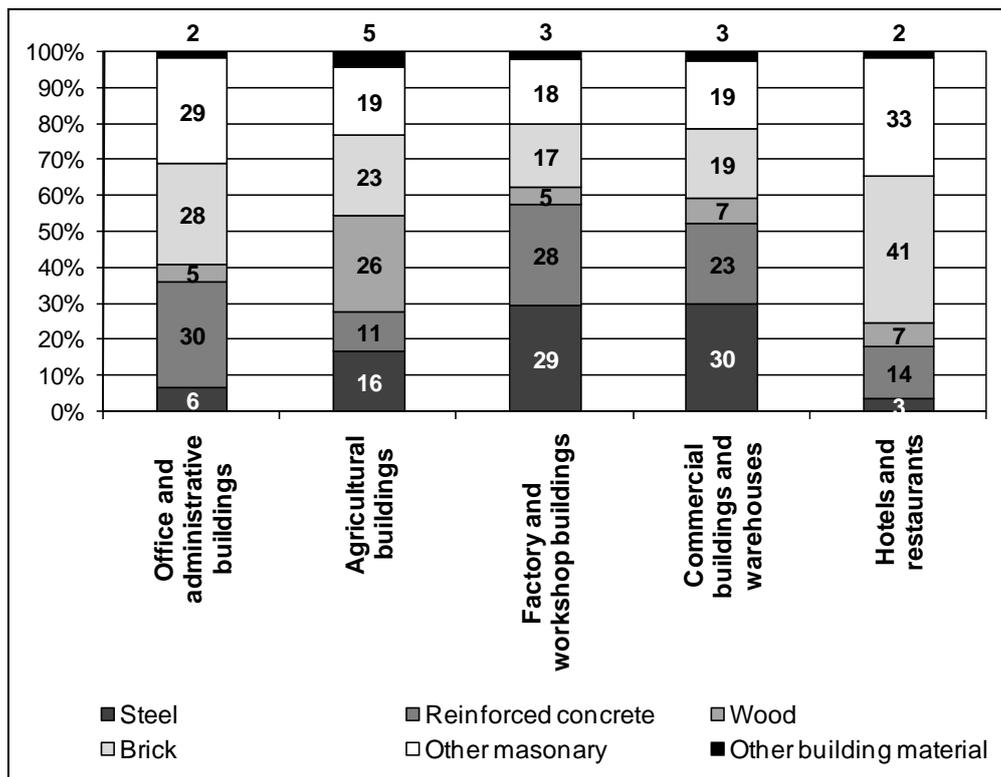
Fig. 3: Building material structure – comparison between building types
