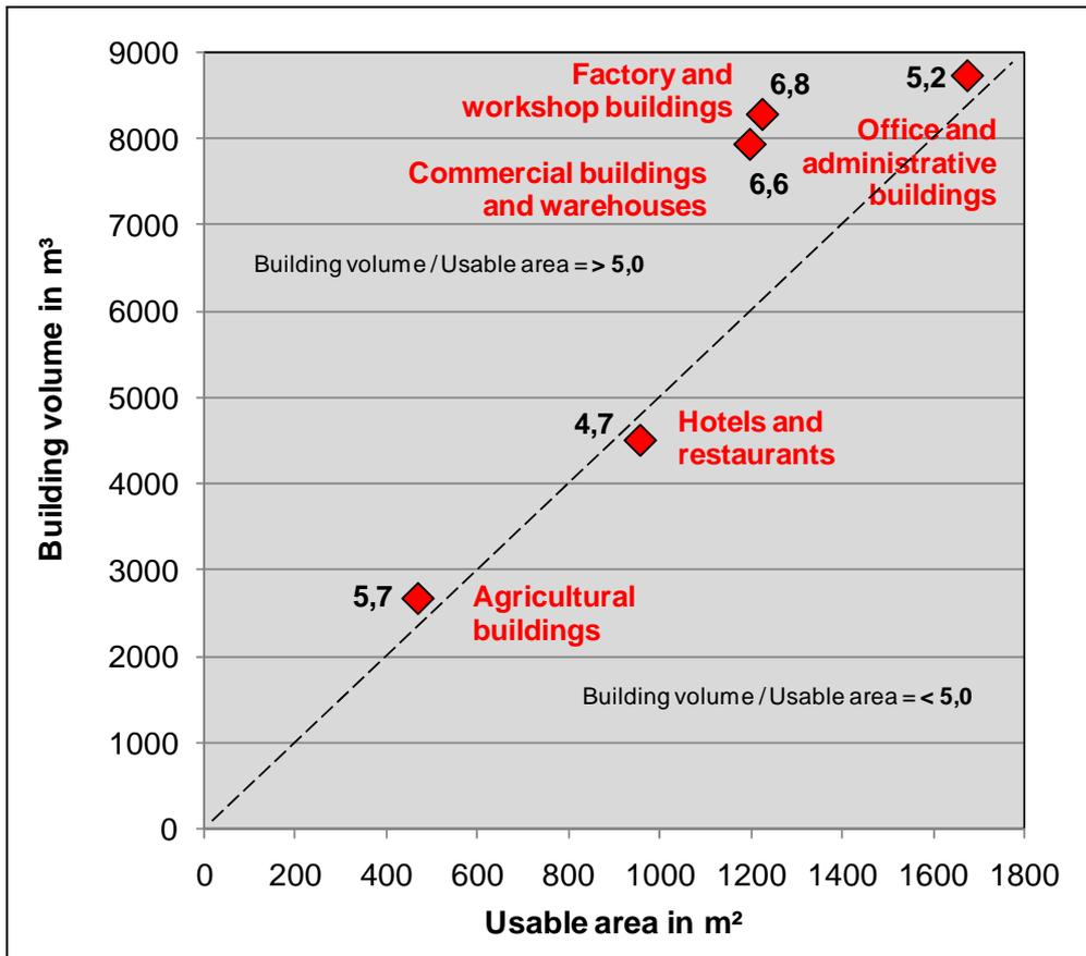
Fig. 1: Usable area and volume per building – comparison between building types
