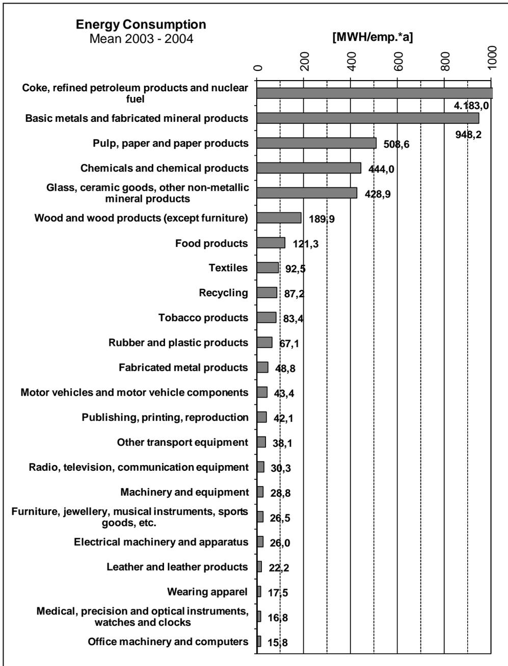
Fig. 4: Energy consumption – comparison between manufacturing sectors
